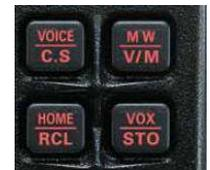
3) Turning the power on while holding the “HOME/RCL” button will both restore adaptation to the factory default settings and clear all memory channels except QMB.
