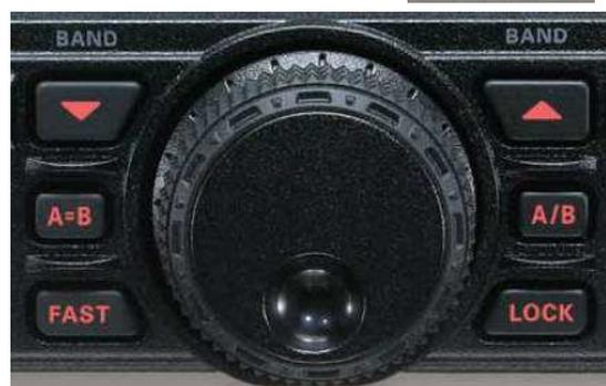
The “MAIN” (large unlabeled) dial (100 steps per revolution) allows fine-tuning of the frequency. The “MAIN” dial is, by default, disabled in AM or FM modes, but may be enabled by adaptation.
