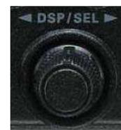
Press the “DSP/SEL” knob to blink the left 3 digits of the frequency display and the “DSP/SEL” knob now moves in 100 kHz increments changing only those digits. Pressing the “DSP/SEL” knob again (or pressing any button or moving the “MAIN” dial) stops the blinking and the “DSP/SEL” knob action returns to the smaller increment size.
