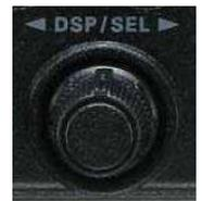
Note: If you make a mistake, after the channel has been turned off, the information is still there. To restore the channel, f-press “MW/V/M” button, select the channel with the “DSP/SEL” knob, press “CLAR”, and press the “MW/V/M” button to confirm.
