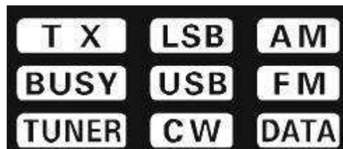
addition, if CW mode, the display also shows whether the injected beat frequency is LSB or USB.
