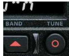
To operate the automatic antenna tuner, t-press the “TUNE” button for one second. The TX will light up during the operation and you might hear the tuner operation for a couple of second. If the operation fails (usually because of excessive SWR), the antenna symbol at the start of the diagram on the display will flash until the tuner is either turned off or run successfully.
