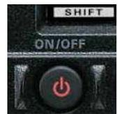
The power switch is also used to reset memory and/or adaptation in the FT-450. Warning: Do not perform any of the first three following steps unless you are prepared to lose information:
