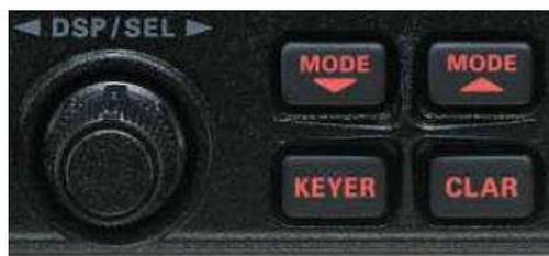
The system will remember the offset value, even when CLAR is turned off. To zero the offset, t-press the "CLAR" button while the clarifier is turned on. The offset will also be set to zero if the "MAIN" dial is inadvertently turned when the CLAR is turned off.
